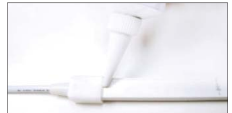
Step 6. Use silicone glue to adhere end cap and front cap.
